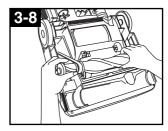
Remove agitator and used belt. Discard used belt.
